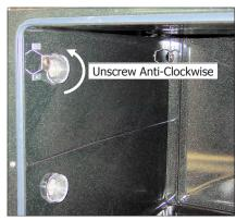
c. Remove seal fitted between lamp glass and holder.
